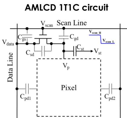
$$\Delta V_p = \frac{C_{gd}\Delta V_{\text{scan}} + C_{sd}\Delta V_{\text{data}}}{C_{gd} + C_{st} + C_{LC} + C_{sd}}$$
