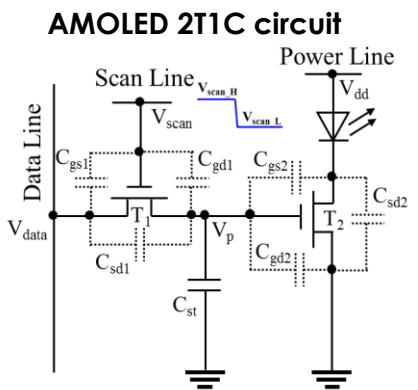
$$\Delta V_p = \frac{C_{gd1}\Delta V_{\text{scan}} + C_{sd1}\Delta V_{\text{data}} + C_{gs2}\Delta V_{\text{OLED}}}{C_{gd1} + C_{sd1} + C_{st} + C_{gs2} + C_{gd2}}$$
